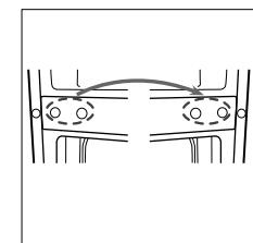
5. Unscrew bottom hinge. Then remove the adjustable feet from both side.
