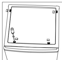
2. Unscrew and remove the hinge.
