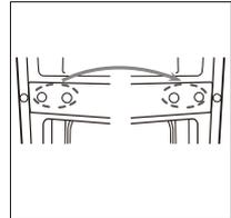
9. Unscrew bottom hinge. Then remove the adjustable feet from both side.
