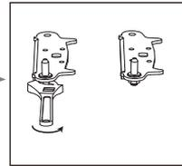
11. Refit the bracket fitting the bottom hinge pin. Replace both adjustable feet.
