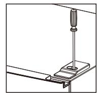
7. Take off the upper door, take out the screw from the middle hinge by cross screwdriver, then take off the lower door.
