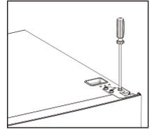
3. Remove the pin with a screwdriver and flip the hinge bracket. Then refit the pin to hinge bracket.
