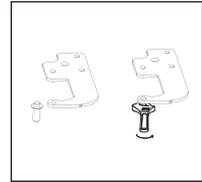
4. Move door switch from right hinge cover to left hinge cover in accessory bag.
