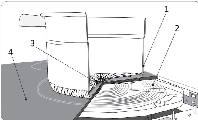
1. Pot with a ferromagnetic bottom
