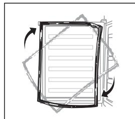
9. Stand up the unit and put the door on the bottom hinge. Make sure the bottom hinge core is inserted in the door hole. Install the door with the upper hinge.
