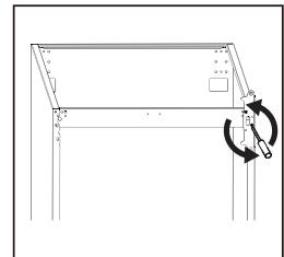
6. Unscrew and remove the bottom hinge pin, turn the bracket over and replace it.
