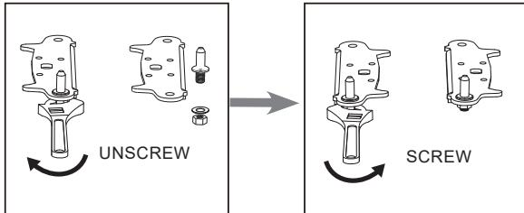
7. Install the hinge at left side and foot base at right side.
