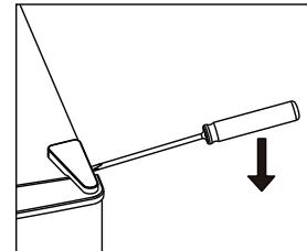
2. Unscrew the top hinge with a philips screw driver.
