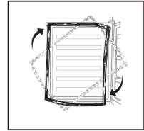
14. Install the lower door, adjust and fix the middle hinge onto the cabinet.
