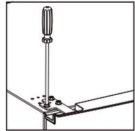
16. Connect harnesses from door and cabinet. Then replace top hinge cover. Before screw the cover, connect terminals of door switch.
