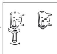
11. Refit the bracket fitting the bottom hinge pin. Replace both adjustable feet.
