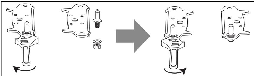
7. Install the hinge at left side and foot base at right side.
