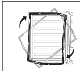
9. Stand up the unit and put the door on the bottom hinge. Make sure the bottom hinge core is inserted in the door hole. Install the door with the upper hinge.
