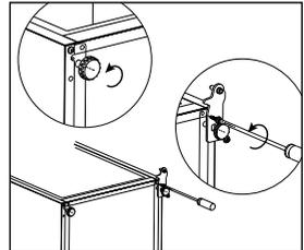
6. Unscrew and remove the bottom hinge pin, turn the bracket over and replace it.
