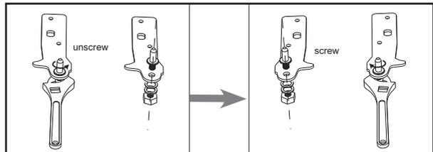
9. Install the hinge at left side and foot base at right side.
