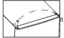
5. Unscrew the middle hinge and then lift the bottom door and put it on a soft pad to avoid scratch.
