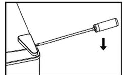
2. Unscrew the top hinge with a philips screw driver.
