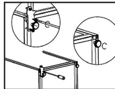
10. Stand up the unit and put the door on the bottom hinge. Make sure the bottom hinge core is inserted in the door hole. Then move the hinge hole cover of bottom door from left side to right side.
