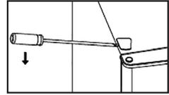
4. Move the core cover from left side to right side. And then lift the upper door and place it on a padded surface to prevent from scratching.
