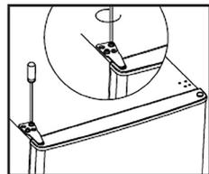
13. Clap in the hinge cover and hole cover on the top of unit.
