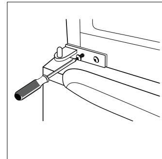
9. Place the upper door back on. Ensure the door is aligned horizontally and vertically so that the seal are closed on all sides before finally tightening the top hinge. Then inert the hinge and screw into the front of the unit.
