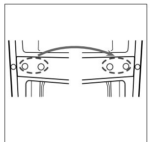
5. Unscrew bottom hinge. Then remove the adjustable feet from both side.
