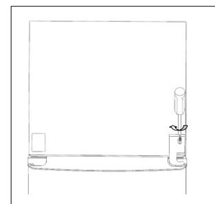
2. Unscrew and remove the hinge.
