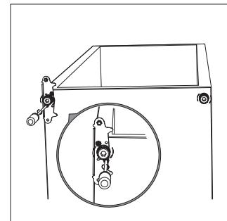
8. Make the middle hinge reverse the direction 180°, the transfer it to the left property position. Make the middle hinge pin in the upper hole of the lower door, then tight the bolts.
